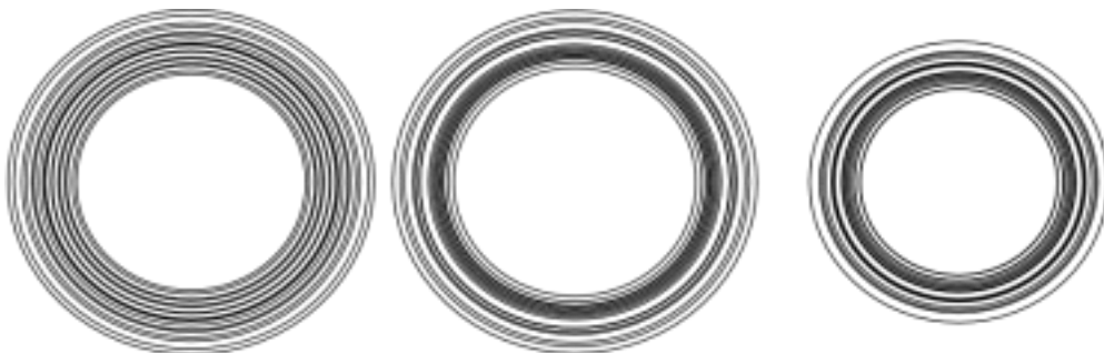
Figure 1. Scheme of the resulting pulleys for ankle (left), knee (center) and hip (right) for the chosen population in [6].
